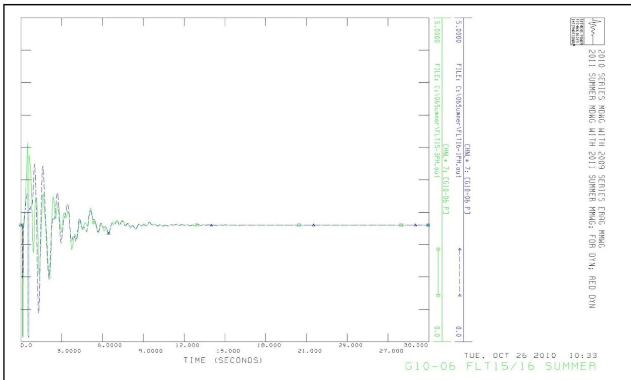
**Figure 5: Response of GEN-2010-006 Combustion Turbine Generator MW Output to FLT15-3PH and FLT16-1PH, Summer Peak**
