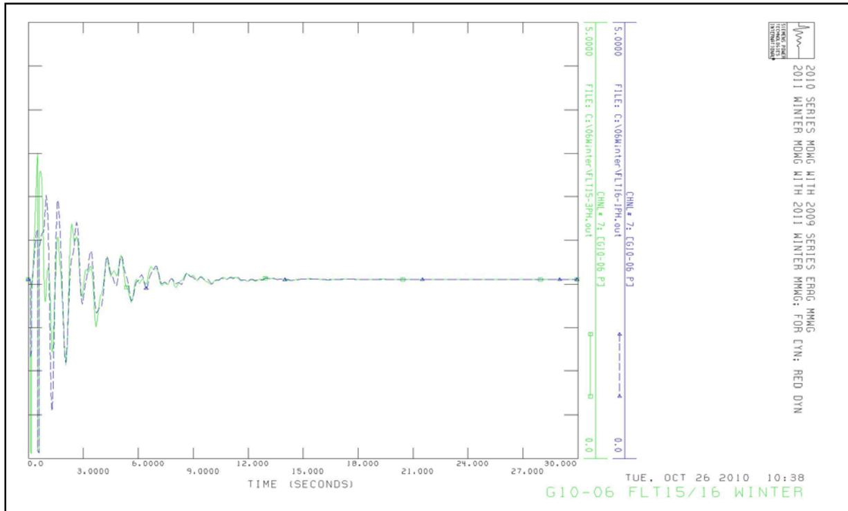
**Figure 6: Response of GEN-2010-006 Combustion Turbine Generator MW Output to FLT15-3PH and FLT16-1PH, Winter Peak**
