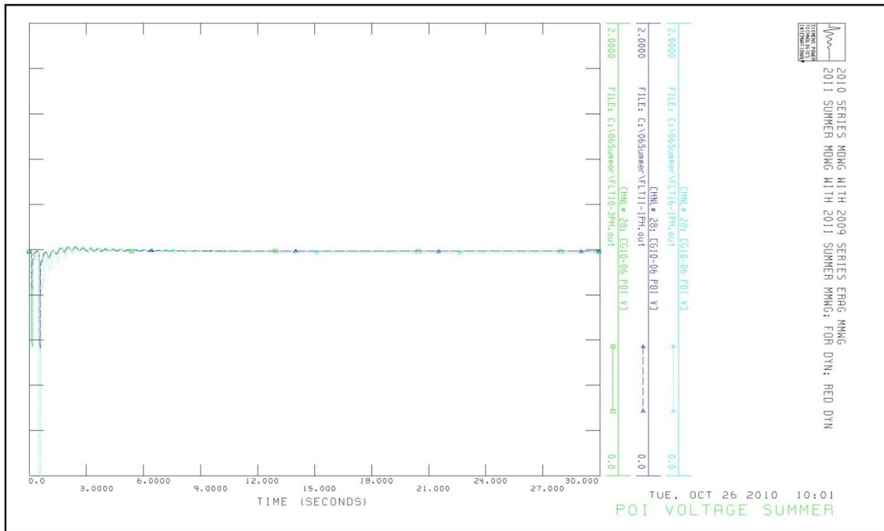
**Figure 3: POI Voltage Recovery for FLT10/FLT11 and FLT16, Summer Peak**
