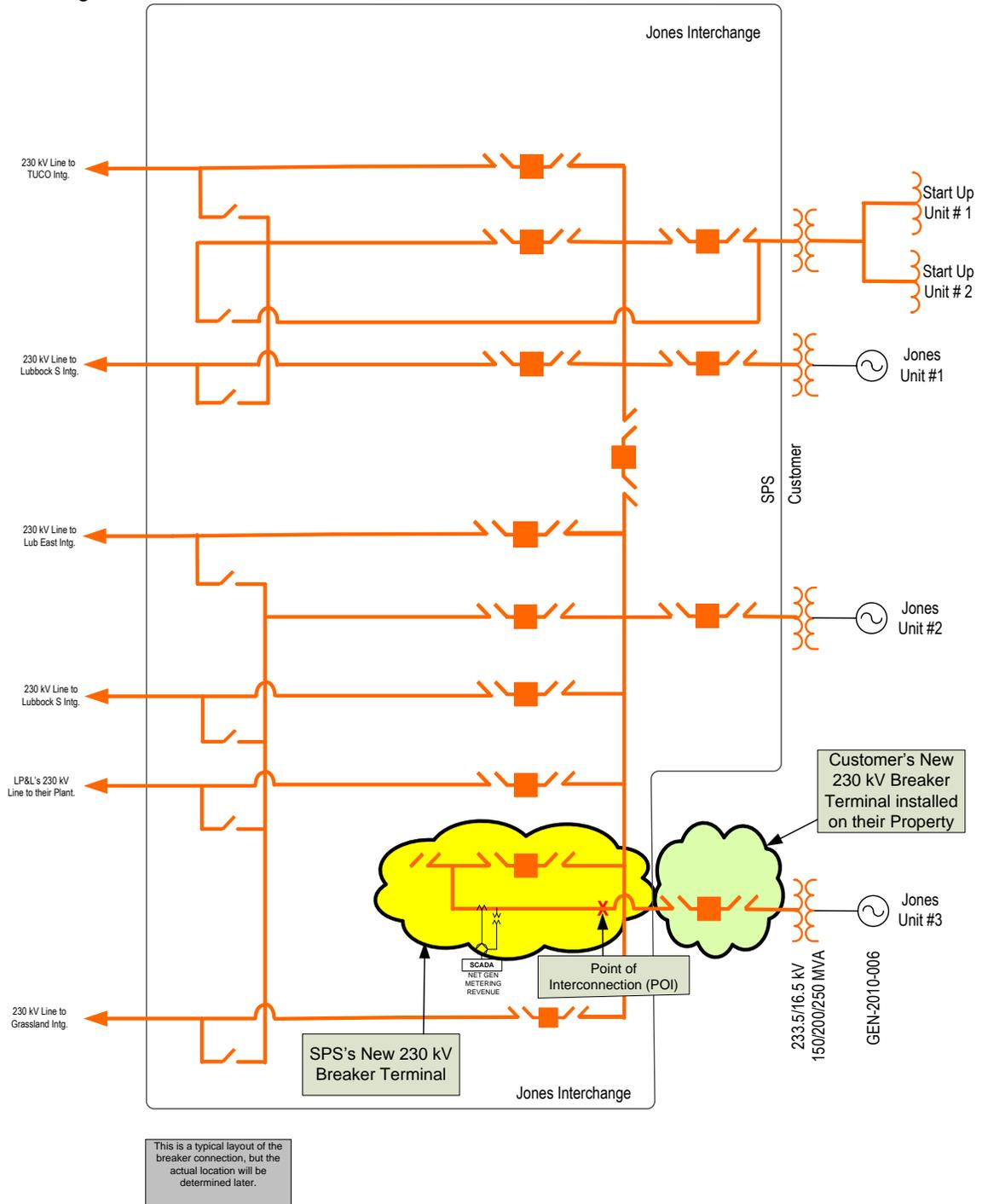
**Figure 1:** GEN-2010-006 Facility and Proposed Interconnection Configuration
