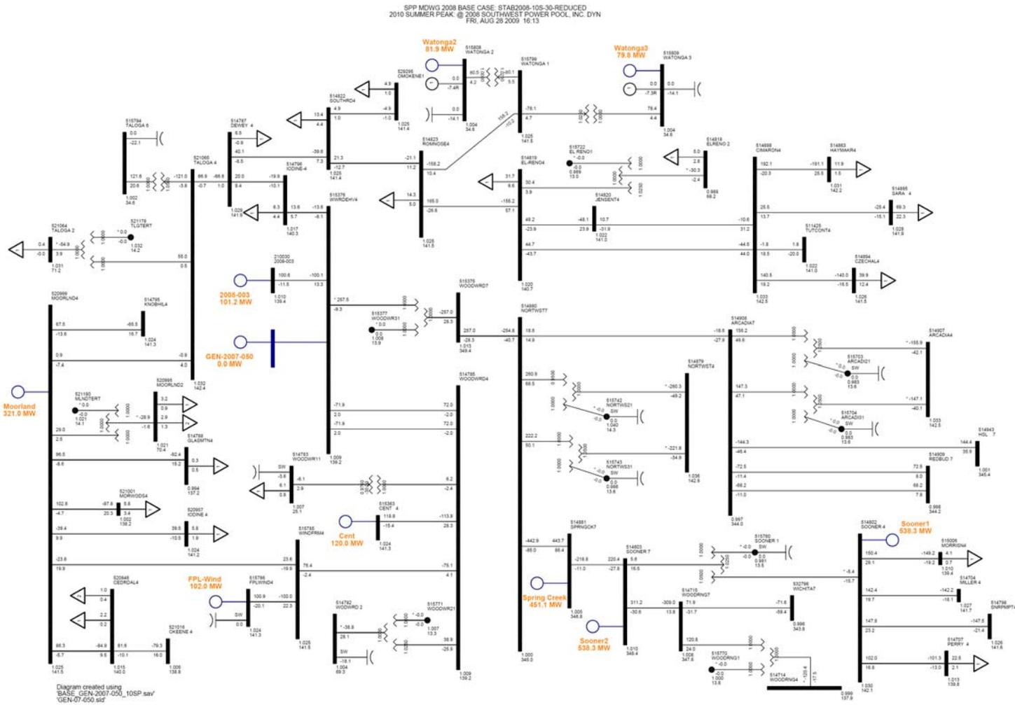
Figure 4-2 One-line Diagram of the local area without GEN-07-050 (2010 Summer Peak)
