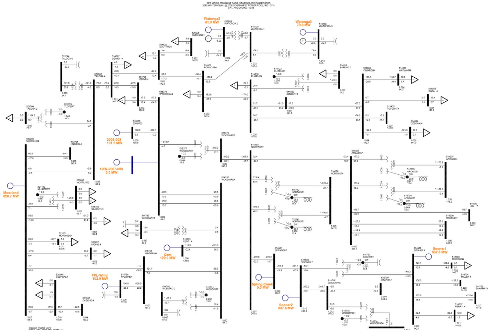
Figure 4-4 One-line Diagram of the local area without GEN-07-050 (2010 Winter Peak)
