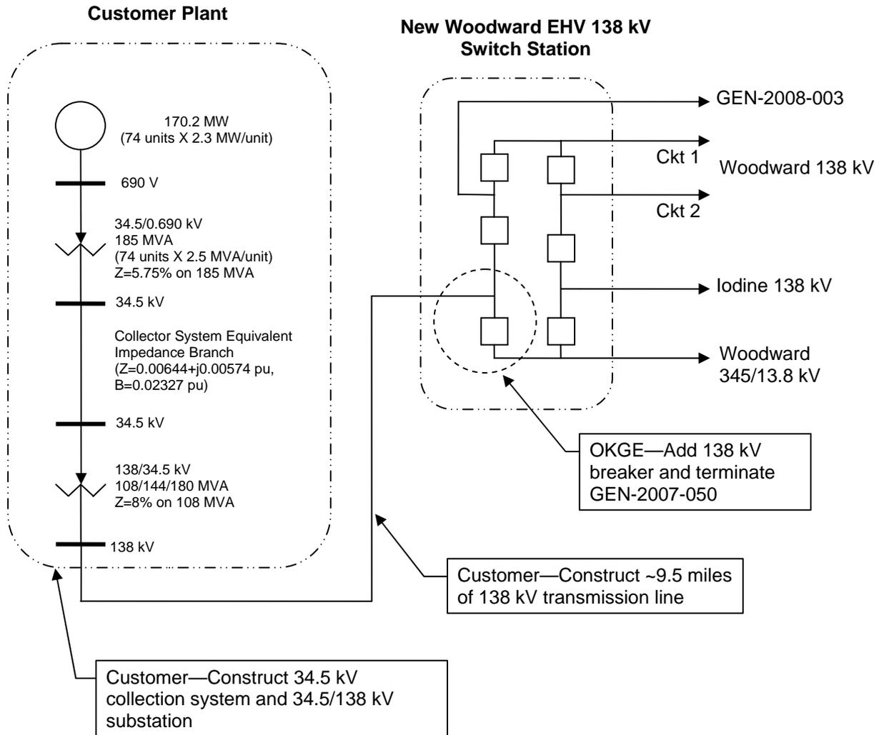
**Figure 1: GEN-2007-050 Facility and Proposed Interconnection Configuration**
