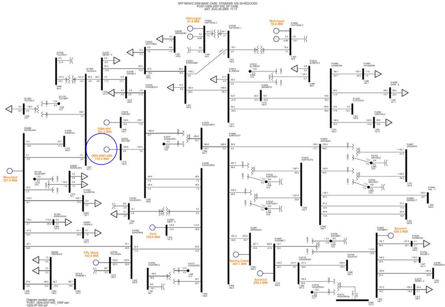
Figure 4-3 One-line Diagram of the local area with GEN-07-050 (2010 Summer Peak)
