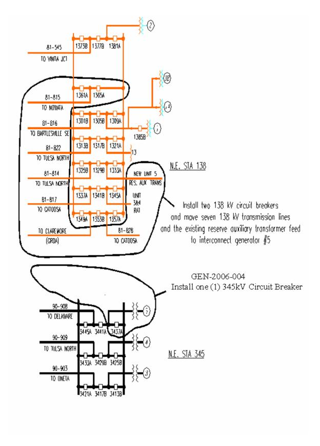
Figure 1: Proposed Interconnection (Final substation design to be determined)
