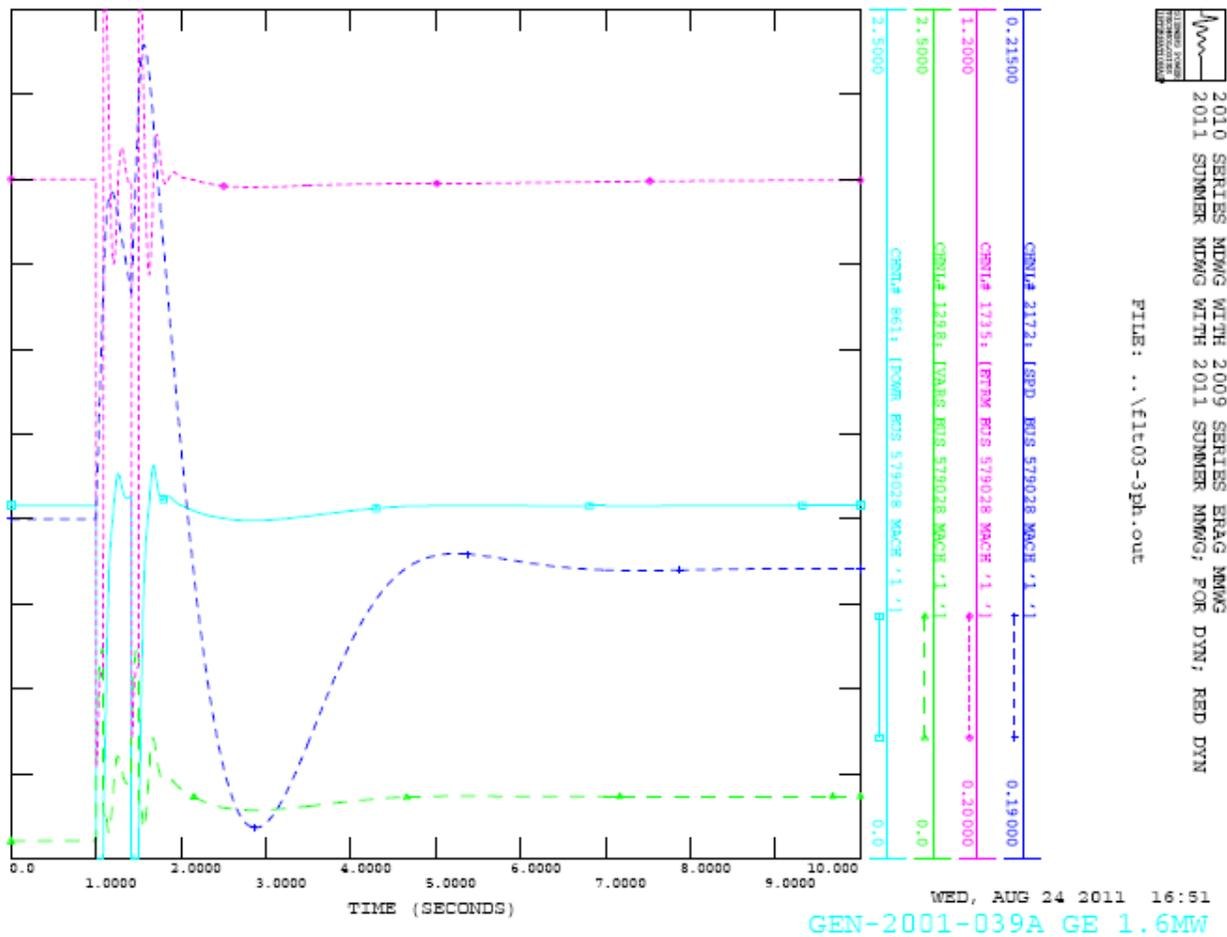
Figure 4-1. GEN-2001-039A Plot for Fault 3 – 3-Phase fault on the GEN-2001-039A Tap to FTDODGE 115kV line, near GEN-2001-039A Tap
