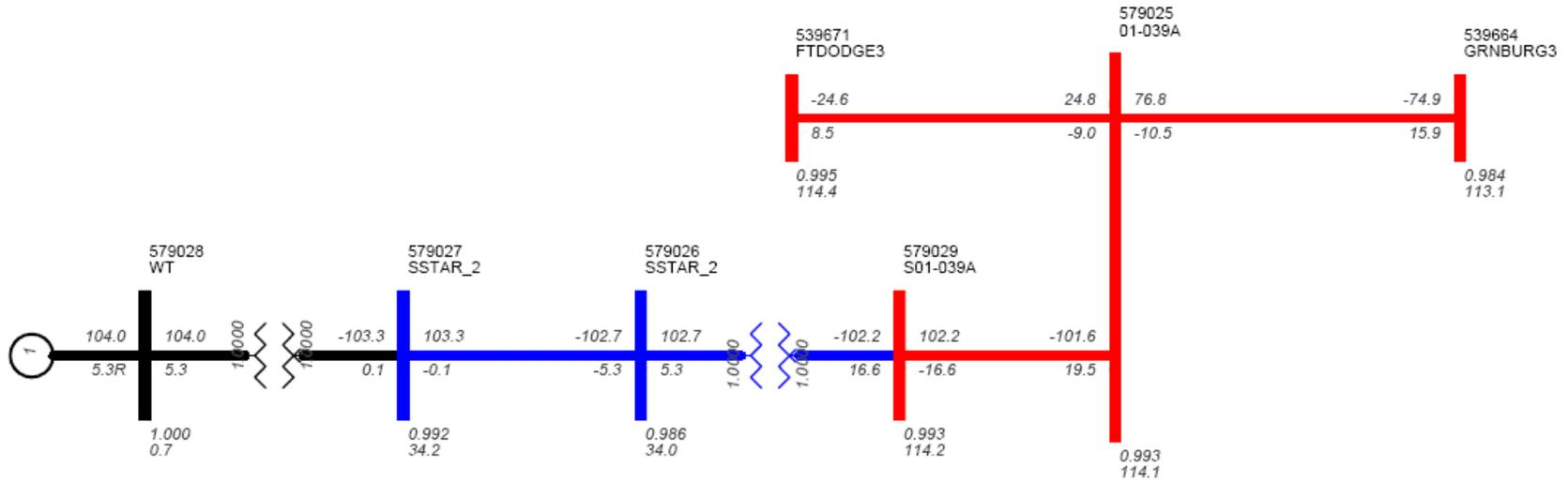
Figure 3-1. Power Flow One-line for GEN-2001-039A and adjacent equipment
