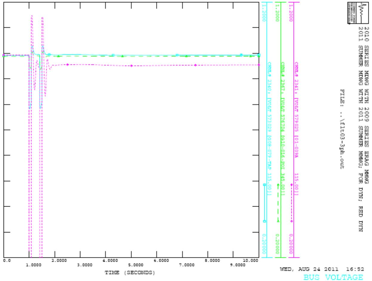
Figure 4-2. POI Voltages for Fault 3 – 3-Phase fault on the GEN-2001-039A Tap to FTDODGE 115kV line, near GEN-2001-039A Tap
